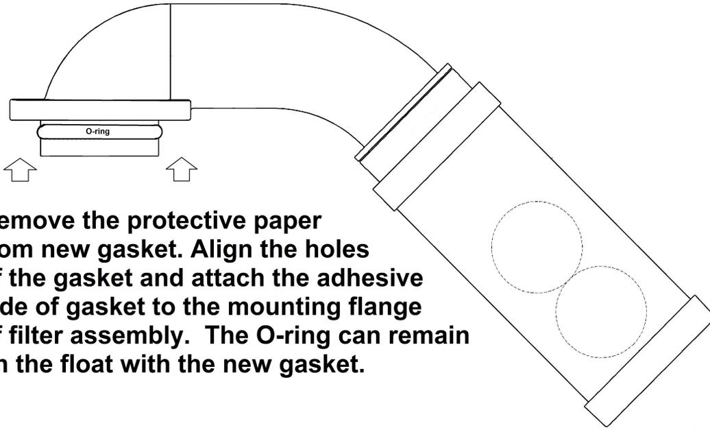
**Remove the protective paper from new gasket. Align the holes of the gasket and attach the adhesive side of gasket to the mounting flange of filter assembly. The O-ring can remain on the float with the new gasket.**
