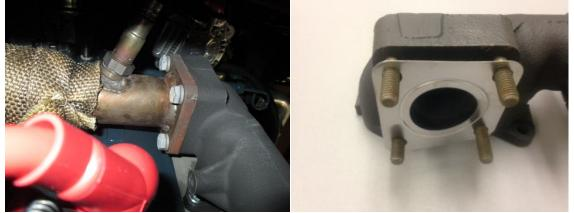
5. Remove 4 nuts on topside, 4 nuts on bottom side of manifold. Save and reuse these nuts on the new exhaust manifold installation.
